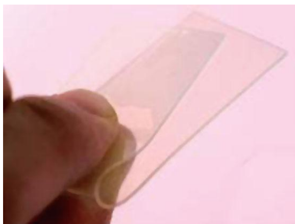
Fig. 7 Transparent, foldable, impregnated nanocomposite based on BC and UV cured acrylic resin[117] (Copyright permission Wiley).
