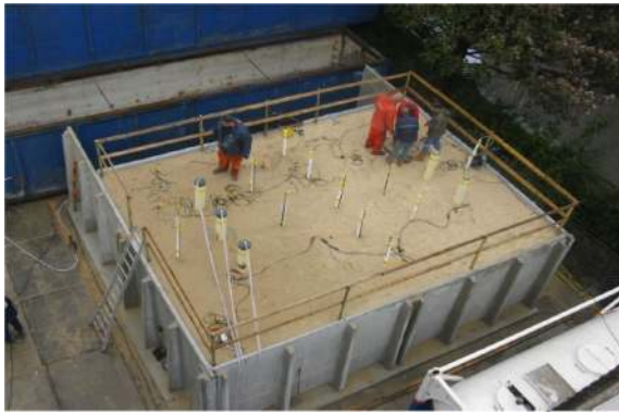
Fig. 4 Upscale studies of 100 m 3 using MICP. (After: [117], with permission from IOS Press)
