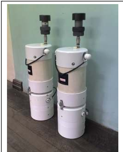
Figure Tanzania_4: Mini-vol samplers for PM 10 determination
