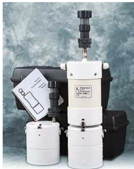
Plate2: Mini-Vol unit.-Typical instrument used for PM10 measurement.
