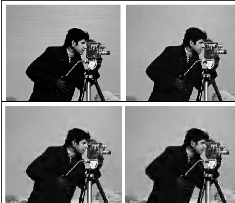
Fig. 9: Simulation results using wavelet transform. (a) Original test image (top left). (b) Compression ratio 12:1, PSNR=32.85 (top right). (c) Compression ratio 31.6:1, PSNR=26.78 (bottom left). (d) Compression ratio 64.25:1, PSNR=23.99 (bottom right).
