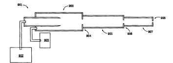
Fig. 23 Focused beam generator schematic making it possible to reduce the spray trace down to 0.8 mm in diameter (Ref 69)
