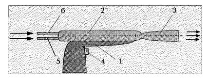
Fig. 6 First portable cold spray gun patented by Nikitin et al. (Ref 16)
