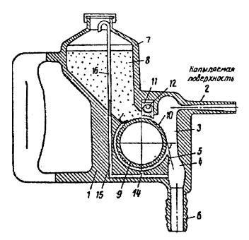
**Fig. 4** First device for applying a coating by cold spray patented in 1986 in Russia (Ref 7)
