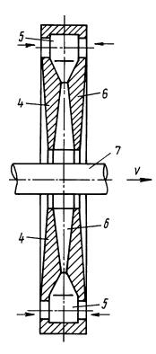
Fig. 12 Device for applying a coating on the outer part of long circular objects (Ref 28)
