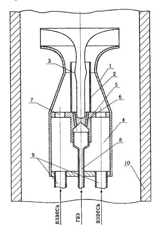
**Fig. 11** Apparatus for applying coating to inner walls of dead and through openings of elongated objects (Ref 27)
