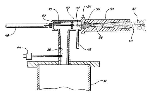
Fig. 17 Kinetic spray apparatus schematic (Ref 51). The system is designed to deposit particles larger than 50 μm in diameter which is outside the range of particle size included in earlier patents
