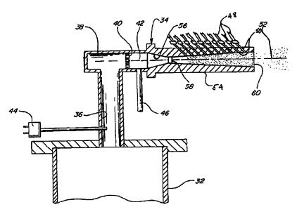
Fig. 20 Low pressure kinetic spray nozzle schematic (Ref 57, 58). The powder particles are injected in the divergent part of the nozzle at a position where the pressure is slightly above atmospheric
