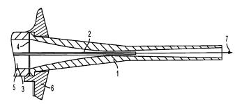
**Fig. 21** Low pressure axial injection powder nozzle schematic (Ref 61). The injection of powder particles is improved by the feeding made on the axis directly in the core of the gas flow
