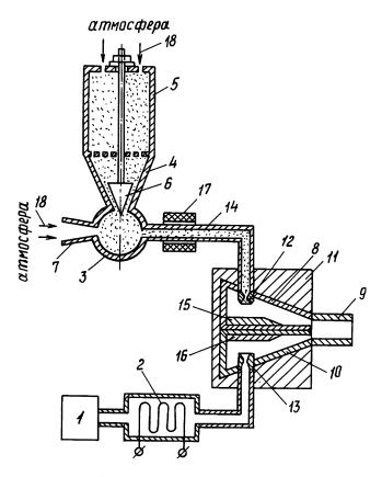
**Fig. 9** Small size nozzle composed of an upper and a lower part generating two flows that are accelerated and superimposed to form a steady flow with particles (Ref 22)
