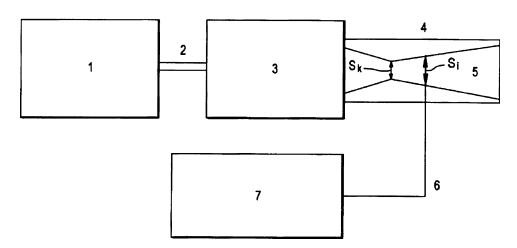
**Fig. 19** Low pressure cold spray system schematics (Ref 14). The claim gives the position in the diverging section of the nozzle where the pressure inside the nozzle becomes below atmospheric and consequently where particle powder can be injected by suction, without pressurized powder feeder
