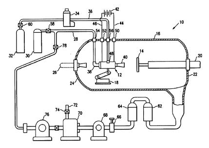
Fig. 22 Vacuum cold spray system schematic patented by Muehlberger (Ref 63). This system makes it possible to reach higher particle velocity with lower inlet gas pressure. The spray process is totally contained allowing for gas recovery and powder overspray collection
