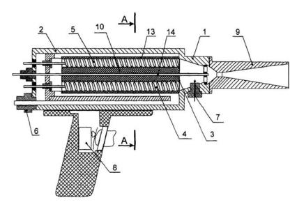
Fig. 7 Spraying unit remotely operated hand tool (Ref 18). The novelty of this invention resides in the capacity of heating the working gas in the spray unit for improved performance
