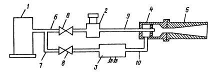
Fig. 5 Cold spray apparatus with separated ducts for preheated propelling gas and for gas-powder mixture (Ref 11)
