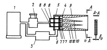
**Fig. 8** A multi gas-powder mixture channels nozzle patented in 1994 for increasing the spray area while limiting the angle of divergence of the supersonic sections to ensure a steady flow (Ref 20)
