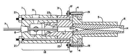
Fig. 16 Redesigned cold spray nozzle minimizing warpage at operating temperatures and improving leak-tight characteristics (Ref 47, 48)
