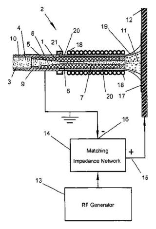
**Fig. 18** Kinetic metallization system schematic (Ref 53). A long friction compensated sonic nozzle is used combined with preheating powder capability
