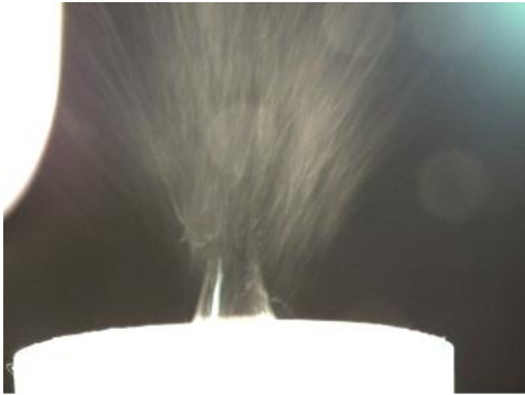
Figure 3. Multiple charged jets from daughter bubble cascades. The multiple jets come from the previous broken bubble, the bubble we see is a new production of the gas supplier
