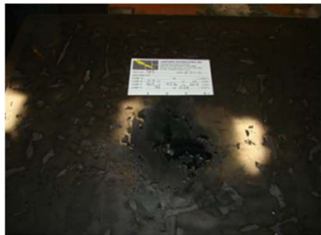
Figure 8: The damage caused by lightning on an FRP [20].
