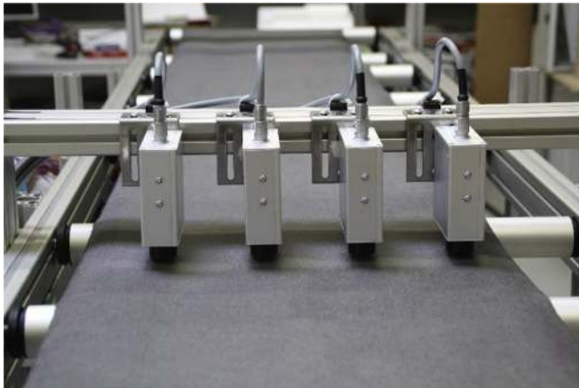
Fig. 14. Prototype EddyCus® Inline for Inline gramature determination by RF EC.
