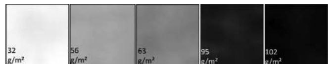
Fig. 12. EC contrast function for Carbon fleece with different weight per area (100 × 100 mm).
