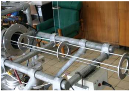
FIGURE 6: Experimental setup of obstacles location along the detonation tube [33].
