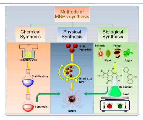
FIGURE 1 | Schematic illustration of the synthesis of magnetic nanoparticles (MNPs) with different methods.
