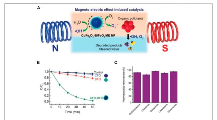
**FIGURE 5 | (A)** Scheme showing magnetoelectric (ME) effect induced catalytic degradation of organic pollutants using core–shell CFO–BFO NPs under magnetic fields **(B)** Catalytic degradation curves obtained for model organic dye, RhB, under 15 mT and 1 kHz magnetic fields **(***n* = 5**) (C)** Removal efficiency of a cocktail of five common pharmaceuticals using the core–shell NPs **(***n* = 4**)**. Copyright 2019, John Wiley and Sons (Mushtag et al., 2019).
