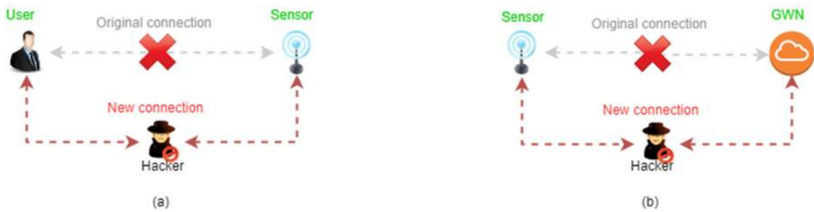
FIGURE 5. Man-in-the-middle attack in IoT network during authentication. (a) User and sensor scenario and (b) sensor and GWN scenario.
