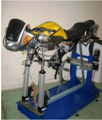
Fig. 9. The developed riding motorcycle simulator by INRETS-UEVE
