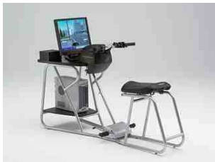
Fig. 3. The Honda SMARTrainer low-cost simulator [7]
