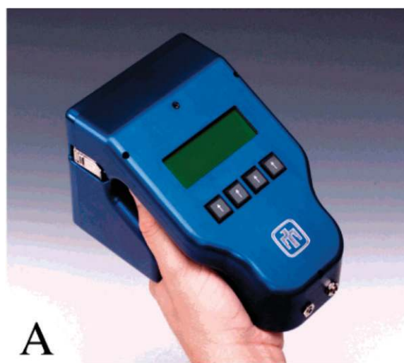
Figure 7. Photograph of the \mu ChemLab hand-held CE system. Reprinted with permission from [95]. Copyright (2005) American Chemical Society.
