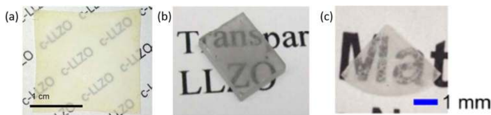
Figure 2. Images of highly dense LLZO material exhibiting varying degrees of translucency depending on the density of defects within the sintered material. (a) Thin film made by tape casting reproduced from Reference 38 with permission from the Royal Society of Chemistry; (b) a bulk ceramic piece processed by pressure assisted sintering reproduced from Reference 39 with permission from the American Chemical Society; and (c) a bulk ceramic LLZO piece exhibiting partial areas of high density made with hot isostatic sintering methods reproduced from Reference 33 with permission from Elsevier.
