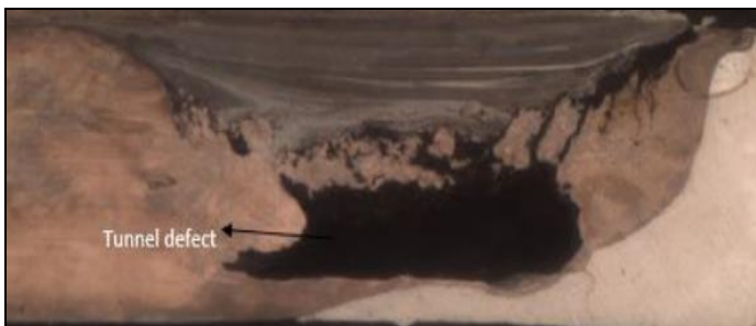
Figure (10): Showing a macrograph image of a FSW with tunnel defect appearance at the bottom toward advancing side in the stir zone when aluminum alloy 5052 on retreating side and stainless steel 304 on advancing side located and joined in FSW with zero tilt tool angle, low rotational speed, and slow weld travel speed. This study made by Chitturi et al. [76].
