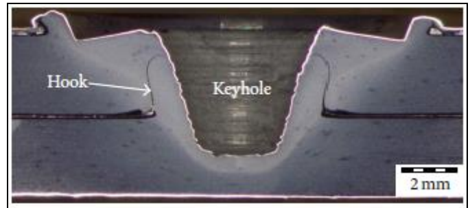
Figure (14): A macrograph of cross-section lap joint with hooking defect observed in Liu et al. study [94], when 2A12-T4 Al alloy was friction stir spot welded.
