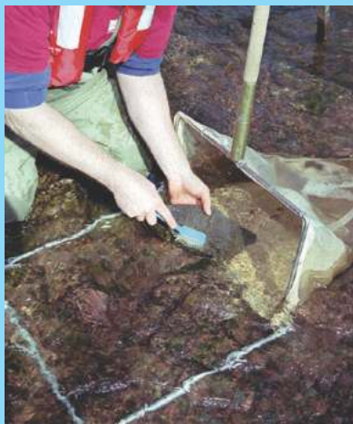
b. Removing attached invertebrates from large cobbles with a hand brush just upstream of the Slack sampler opening.
