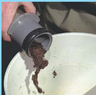
d. Transferring the discrete collection into a 19-L (5-gal) plastic bucket.
