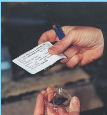
e. Label placed on petri dish containing subsample filter and then frozen in a plastic bag.
