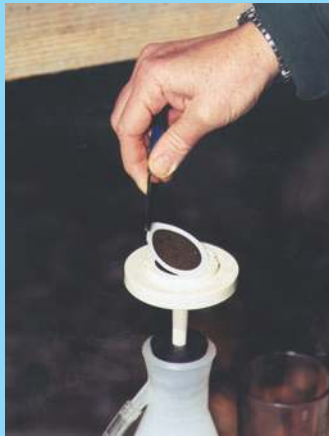
c. CHL A or AFDM subsample filter removed from filter base with forceps.
