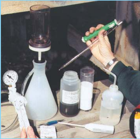
a. Apparatus used to filter microalgal sample components: hand-operated pump, Erlenmeyer flask, tubing, filter funnel and base.
