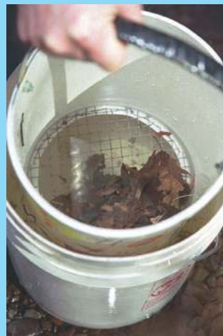
e. Rinsing pieces of large organic material using a dual wash bucket.
