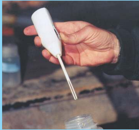
b. Homogenizing the microalgal sample component with a battery-powered stirrer.
