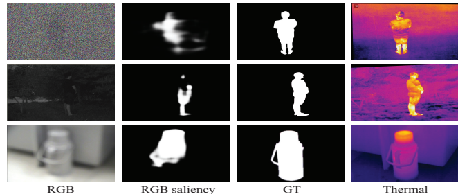
Fig. 1. Saliency maps generated by RGB-based salient object detection model for some images in complex scenarios (occlusion, lack of illumination and low contrast) and their ground truth annotations. The last column shows the corresponding spatially aligned thermal images to the RGB images.
