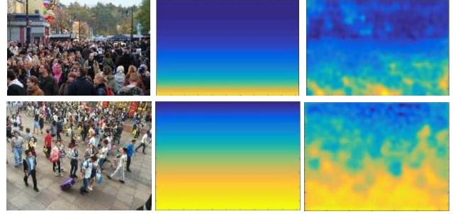
Figure 3: Perspective samples from SHA and SHB [47]. In each row, the left column is the original image, middle column is the GT perspective map using (6) while the right column is the estimated perspective map by PACNN. Blue in the heatmaps indicates small perspective values while yellow indicates large values.
