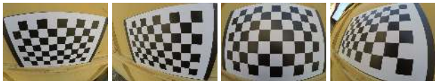
Figure 3: Images of a calibration pattern recorded by a Go-Pro camera in medium and wide field-of-view mode.
