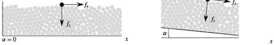
FIGURE 1. (Colour online) Schematic slope influence on a particle at the top of the granular bed at rest.
