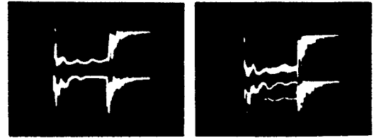
Fig. 9. Forward and reflected RF wave shapes: a) normal, b) during breakdown.
