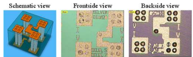
Fig. 3. Schematic drawing and final front and back-side metal patterning for Kelvin structure.
