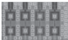
Figure 4: Oscillator tuned with switched capacitor; layout of RF switch FET
