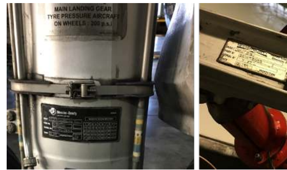
Fig. 2 Nameplate-based traditional aircraft parts marking: MLG main fitting (left), and lock stay (right)
