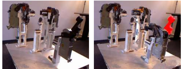
Figure 13: Live meshing allows to quickly create a textured meshed model of an object for visual discrepancy check (see supplementary material video).
