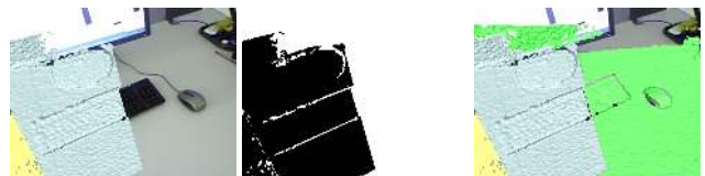
Figure 5: Determining the contribution of a potential new keyframe. The reconstruction is rendered from the current camera viewpoint (left), creating a binary mask (center) set at rendered pixels. New geometry from the potential keyframe is only added to the reconstruction when there either was no geometry at all (right) or in case the rendered geometry is further than a specified distance away.
