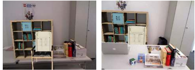
Figure 12: AR-based virtual furniture trial: correctly handling the occlusion thanks to the proposed parallel tracking and meshing of the environment makes the AR visualization much more realistic. While the camera moves, the camera motion is estimated and the environment model is updated (see supplementary material video).
