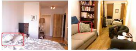
Fig. 1. Some hard samples of semantic segmentation only by RGB image. Left: pillows on a bed with similar color of the bed. Right: cushion on a sofa with similar color of the sofa.
