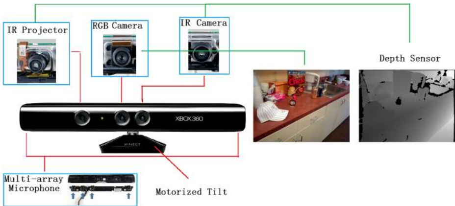
Fig. 1 Illustration of the structure and internal components of the Kinect sensor. Two example images from RGB and depth sensors are also displayed to show their differences
