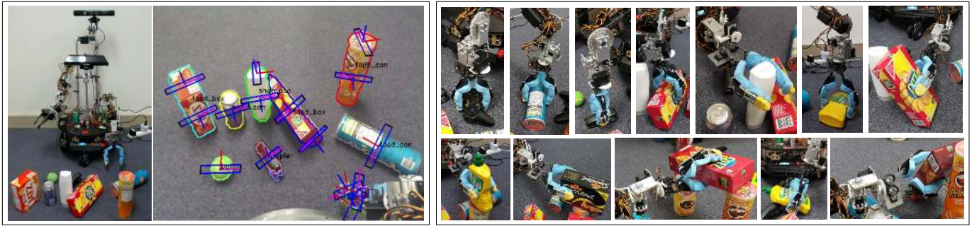
Fig. 13. Left: Visualization of our robotic experiment setup (where objects are placed in front of the robot in different orientations and locations, and the task of the robot is to pick a target object selected by the human operator), and the output of the proposed framework in terms of segmented objects, their predicted class labels and estimated grasp rectangles (each with a fixed height of 3 cm). Right: Examples of robotic grasping. Figure best viewed in color.
