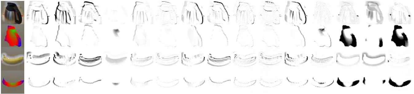
Fig. 5: CNN activations for sample RGB-D frames. The first column shows the CNN input image (color and depth of a pitcher and a banana), all other columns show corresponding selected responses from the first convolutional layer. Note that each column is the result of the same filter applied to color and pre-processed depth.
