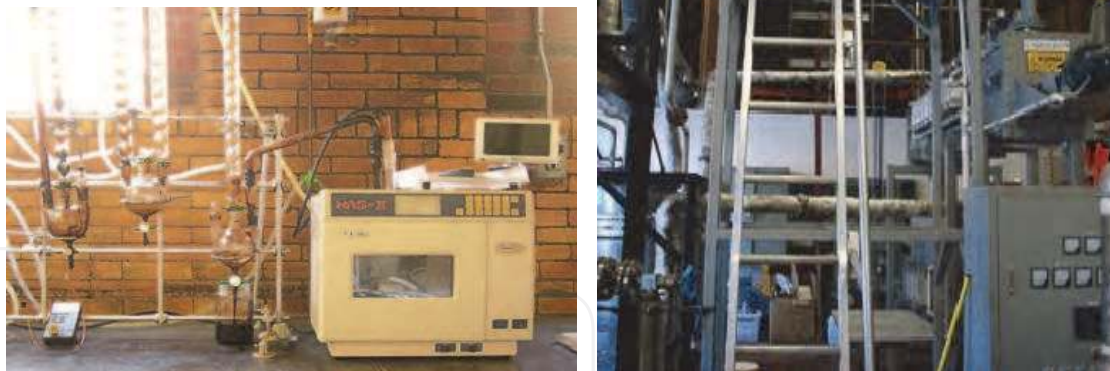
Fig. 1. Batch and continuous microwave assisted pyrolysis (Courtesy: Dr. R. Ruan, University of Minnesota, MN, USA)
