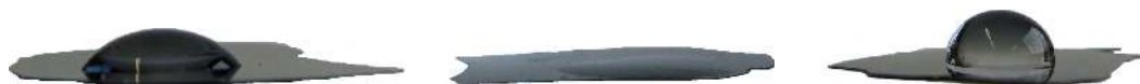
Figure 3.4.: Illustration of the impact of the surface chemistry on the wettability of a substrate elucidated by photographs of water droplets on a planar surface-modified silicon substrate. (left): Silicon as prepared: \theta_0 \approx 50^\circ . (middle): Silicon after 23 h chemical oxidation in \text{H}_2\text{O}_2 : \theta_0 < 10^\circ . (right): Silicon after 23 h chemical oxidation in \text{H}_2\text{O}_2 and subsequent silanization in \text{Si}(\text{CH}_3)_2\text{Cl}_2 : \theta_0 \approx 90^\circ . Courtesy of Anke Henschel, Saarland University, Saarbrücken, Germany.
