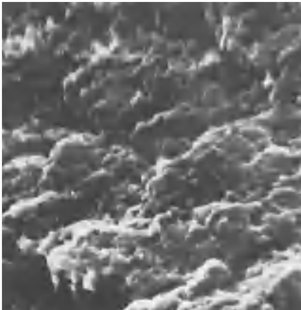
Figure 2. Stereoscanning electron microscopic picture of the fracture surface of a sample of suspension PVC extruded at high shears, at 190°C. Sample fractured at liquid N 2 temperature.
