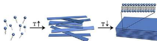
Figure 16. Illustration of structural transition of surfactant in ionic liquid as a function of temperature [Reprinted with permission from ref 201. Copyright 2016. John Wiley and Sons].
