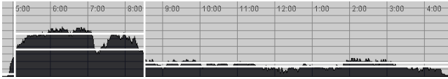
Figure 2. Graph of percent-active levels for Mondays at home showing segment boundaries (vertical white lines) and thresholds (horizontal white lines). Candidate two-sided transitions occur where the percent-active level crosses the thresholds.
