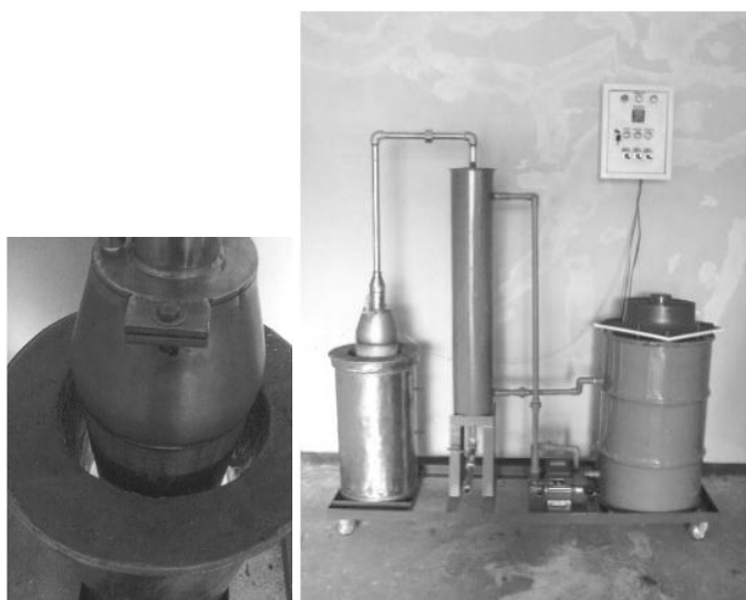
Figure 1. The reactor pyrolysis for producing rice husk biochar
