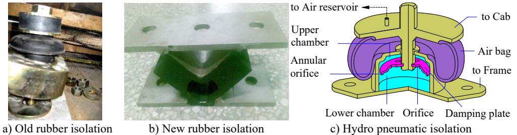
Fig. 1. Structure models of cab isolation systems
