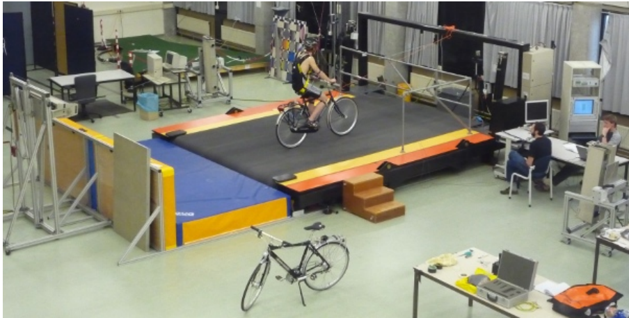
Figure 1: The 3 \times 5 m treadmill at the Vrije Universiteit Amsterdam.
