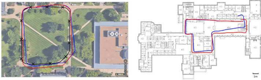
Fig. 6. Overlaying the trajectories with the online digital map (from Google Maps) or the floorplan image with the estimated scale. The red line marks the trajectory given by the Tango system and the blue line marks the trajectory given by our system. The accuracy of the Tango system degrades at outdoors in our experiments, so we manually drew the actual walking path with the black line at the left.
