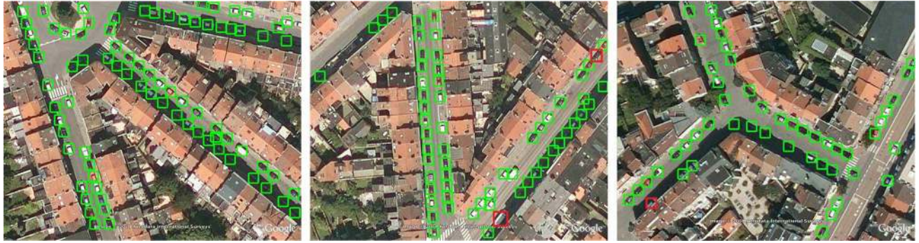
Figure 4. Some example detections (true positive in green, false negative in red) by using our RI-CNN features with a linear SVM.
