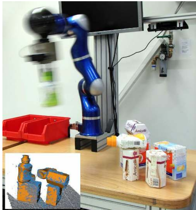
Fig. 14. The setup of the vision-based grasping experiments. The robot has grasped a green soda club bottle and is about to put it in the further red bin. The Kinect sensor can be seen in the upper right corner. In the lower left corner, the range image and the recognized models are shown (before the bottle has been taken away) from a viewpoint close to the one of the sensor.
