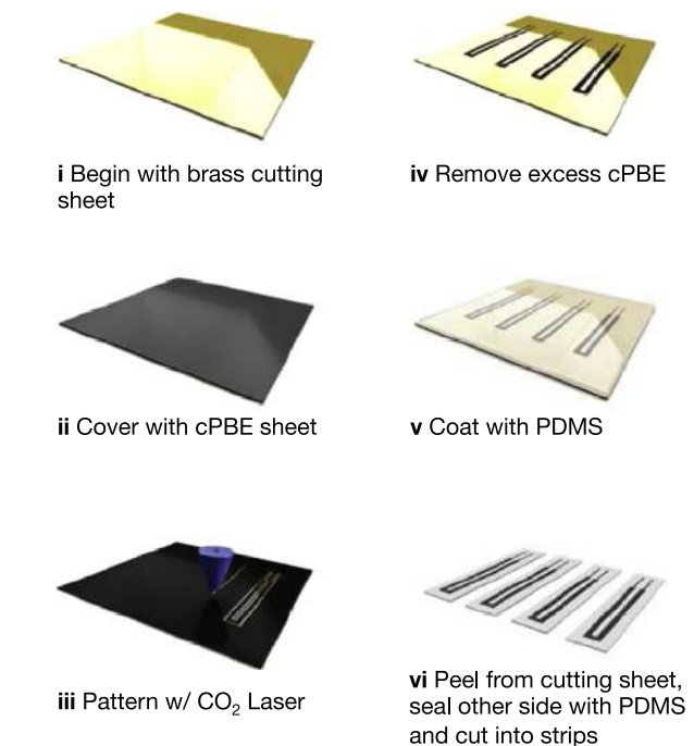
Figure A1. Steps for fabrication: (i) start with a flat cutting substrate, (ii) cover with a layer of cPBE, (iii) pattern with a CO 2 laser, (iv) remove excess material, (v) seal with PDMS, (vi) pattern edges and release.
