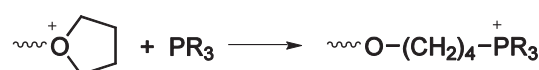
Figure 29. Reaction of the CROP growing chain ends with a phosphine to allow quantitative analysis.
