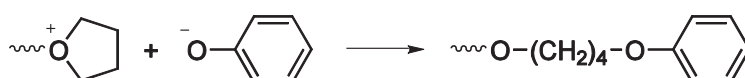
Figure 28. Termination of CROP by phenolate to allow quantitative determination of the growing chains.
