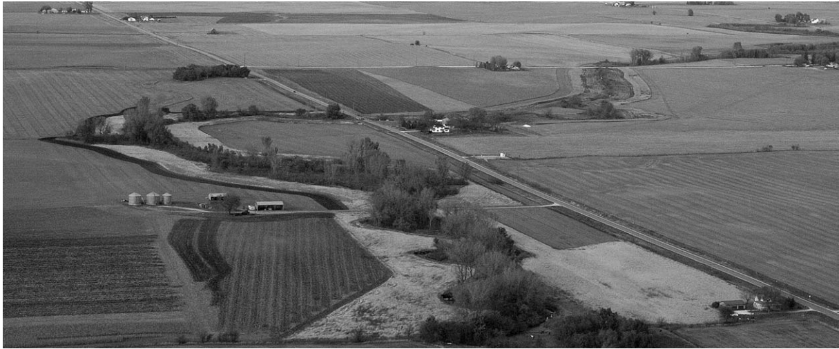
Figure 6. Examples of buffers placed outside the meander belt of the stream and smooth buffer borders to accommodate efficient farming of the upland crop fields. Areas within the meander belt are also planted to a variety of species to provide diverse wildlife habitat.
