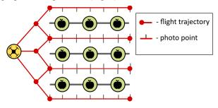
Fig. 3. Flight trajectory of UAV for orchard monitoring.
