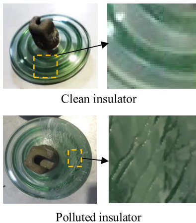
FIGURE 3. Clean and polluted glass insulator.
