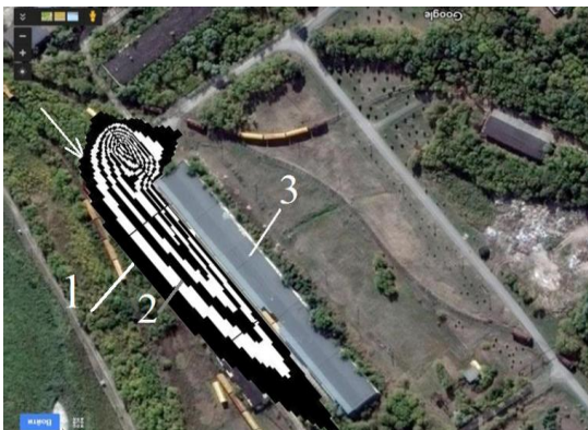
Fig. 5. Zone of thermal pollution (isotherm) near industrial building, t = 32\text{ sec} : 1 – T = 103^{\circ}\text{C} ; 2 – T = 240^{\circ}\text{C} ; 3 – industrial building
