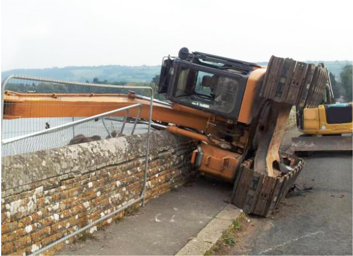
Figure 2 – Excavator overturn example
