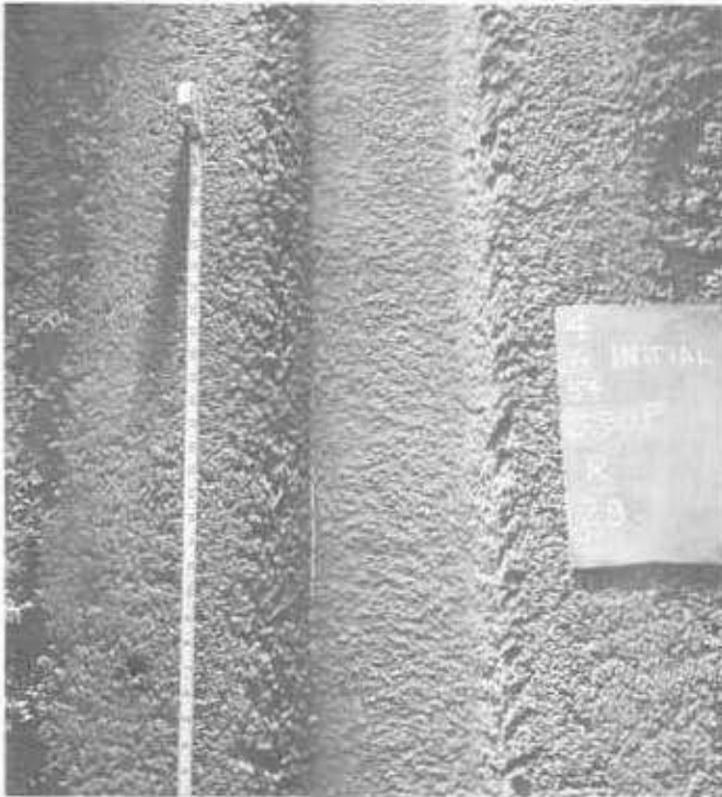
FIGURE 53.—Initial channel molded in flume bed (April 6, 1954, run 29, 3:30 p. m.)
