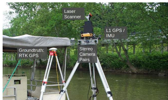
Fig. 13 Surrogate data collection system at the test site on the Allegheny river. Here we see the GPS, IMU, lidar and stereo camera pairs (one temporary COTS unit and the other a lightweight in-house device). There is also a high-end, heavy GPS unit that we use to groundtruth the experiment
