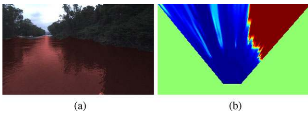
Fig. 7 Local 2D River Mapping: (a) Image with the detected extent of the river (thresholded at P_{river} = 0.5 ) overlaid in red. (b) The same detected extent of the river projected into a top down view. Blue regions are part of the river and red regions are the shore. The surrounding green area is unobserved in this image as it lies outside the viewing frustum (Color figure online)
