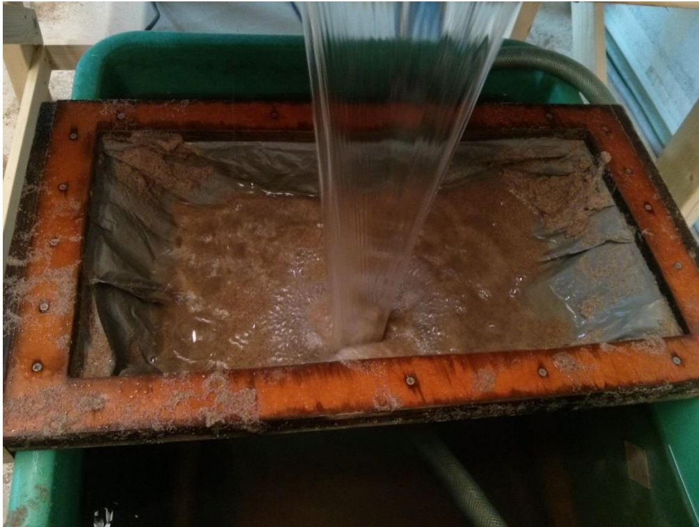
Figure H.9 – Sieve at the downstream end of the flume supported by water basin
