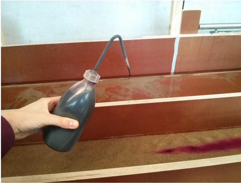
Figure H.23 – Dye in flask that is added to the water flowing in the main channel
