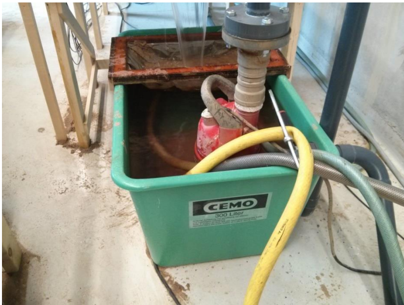
Figure H.10 – Water basin at downstream end of the flume. Green pipe is for water supply from the ball valve. Water that is sucked to the discharge pump flows through the yellow pipe. Water flowing out of the discharge pump goes through the brown pipe and lies in the water basin to keep any leakage of the connection to a longer green pipe (right in figure), that reaches up to the upstream end of the flume, inside the basin. The grey pipe (right in figure) attached to the water basin is used to drain water that exceeds a certain water level to prevent the basin from flooding and to keep the
