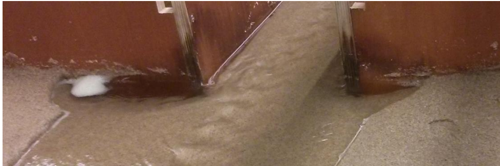
Figure 4.6 – Scour holes in test R13 after 1.5 hours. The flow is from bottom to top of the figure.
