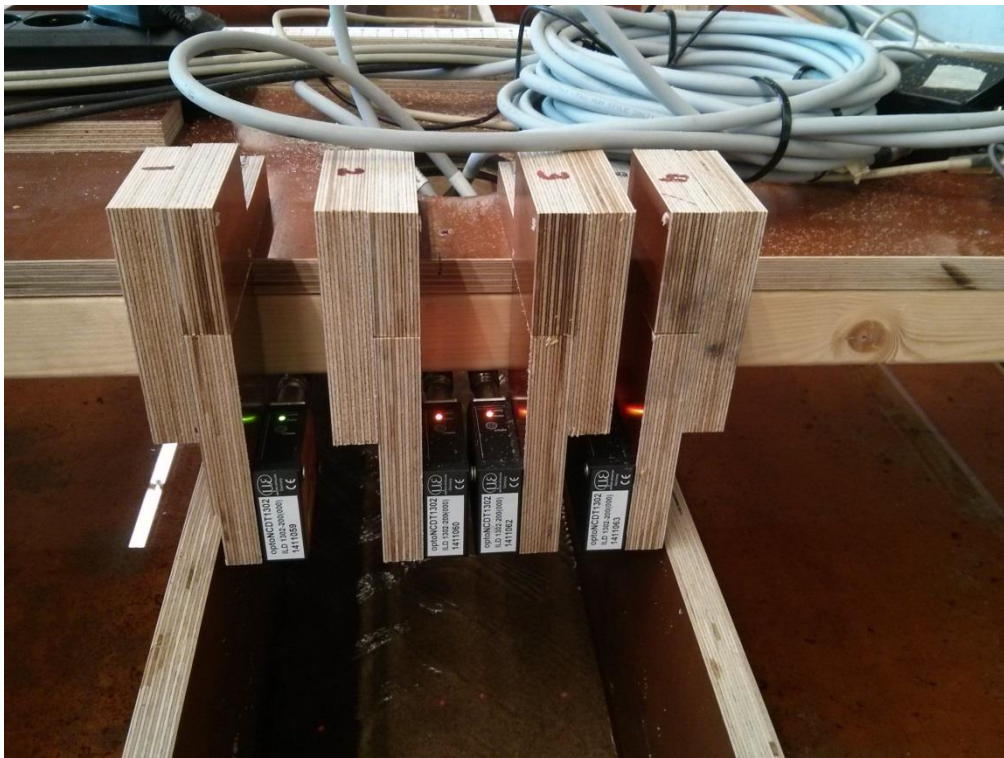
Figure H.14 – Four lasers fixed on platform. Laser number 1, 3 and 4 measure the bed profile in longitudinal direction. Laser number 3 is not in use.
