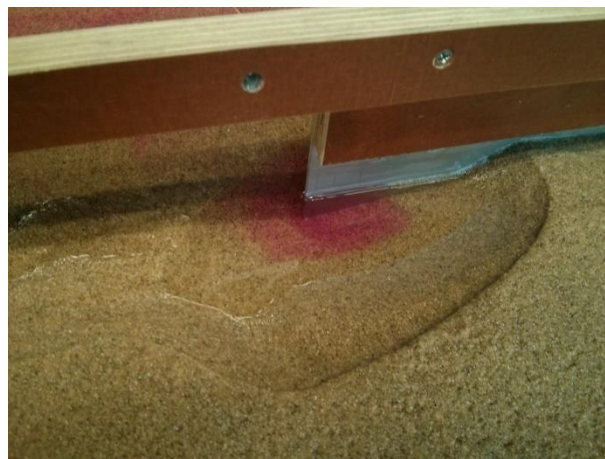
Figure 4.5 – Scour hole in final bed topography of test R01 at the downstream end of the widened section. Red dye indicates deep bed profile.
