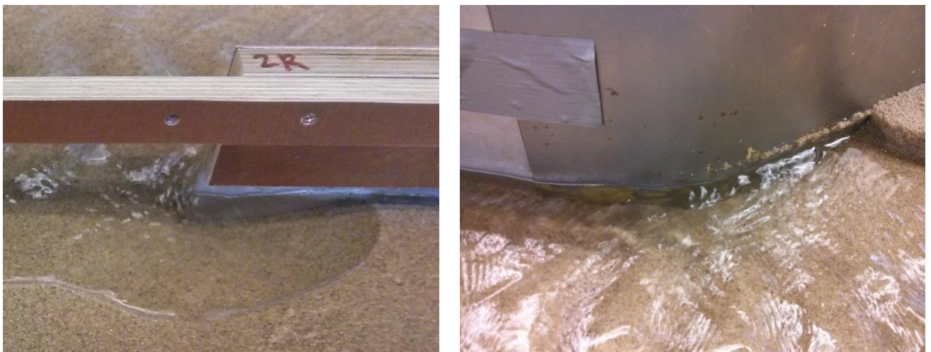
Figure 4.7 – Scour hole in test R01 (left) at the straight bank protection with a diameter of 12 cm and a depth of 3,5 cm (flow from left to right). Scour hole in test R14 (right) at the curved bank protection with a width of 4 cm and a depth of 3 cm (flow from right to left).
