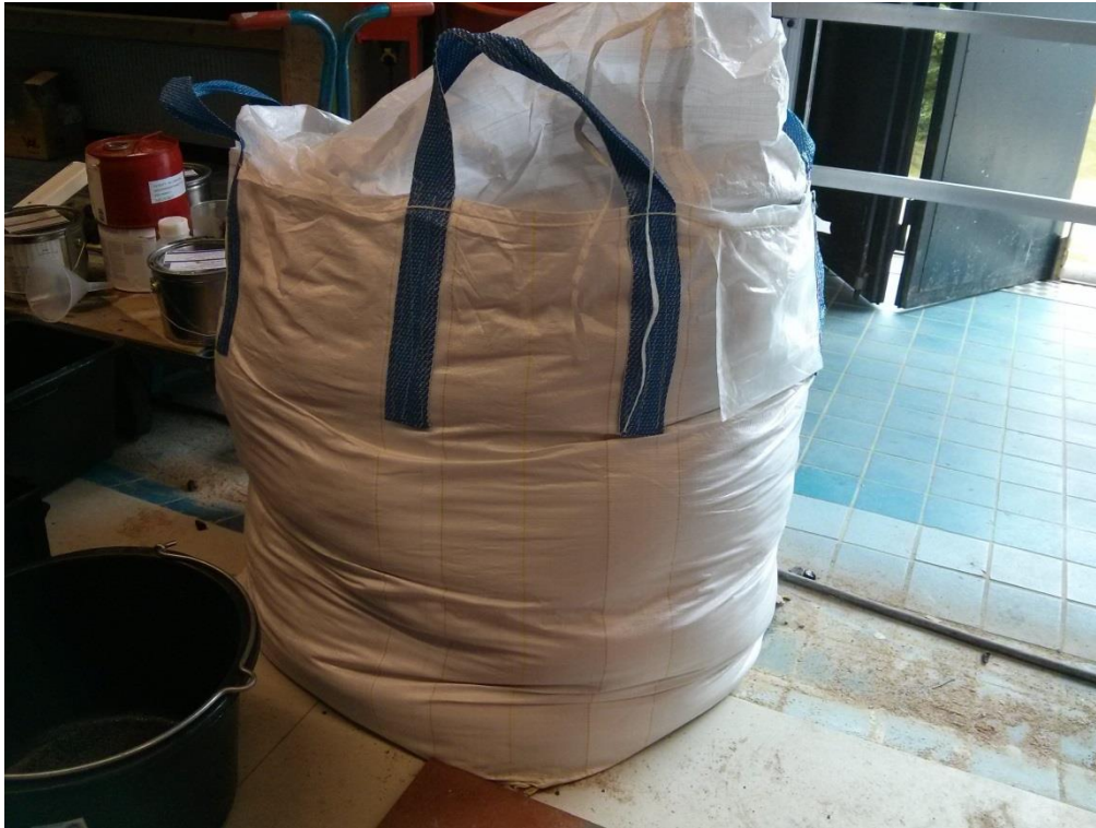
Figure H.7 – Bag of sediment used for the sand-bed in the main channel and filling the sediment feeder
