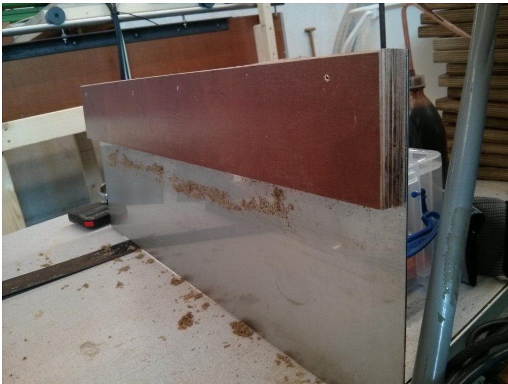
Figure H.4 – Removable bank protection of main channel made out of steel (1.5 mm thick) and wood (2 cm thick) with length of 60 cm and height of 23 cm.
